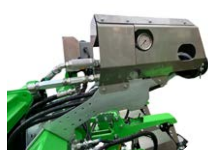
Hydraulic system for the control of the side shifter and the in row hoes
